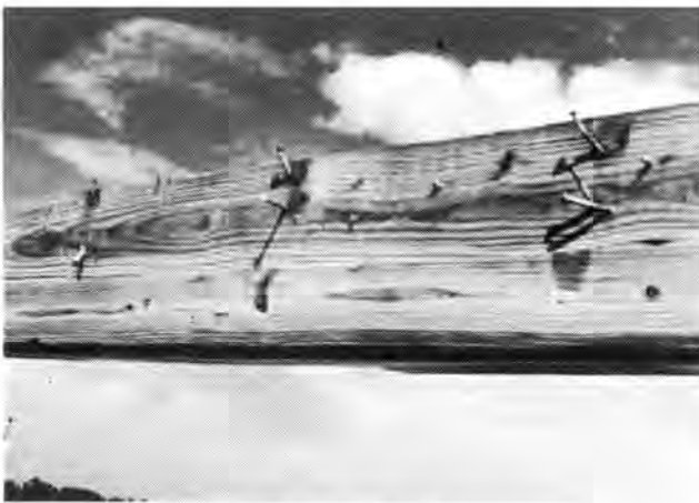
Figure 4.26. Toe Nailing Provides Limited Pull-Out Resistance
