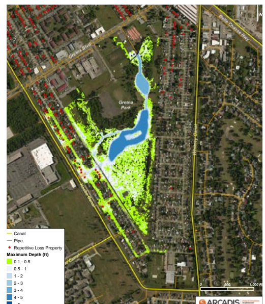
25-year storm modeled flood conditions (above) and with Hero Canal sheet pile wall, flap gates &amp; extra storage in City Park (below)
