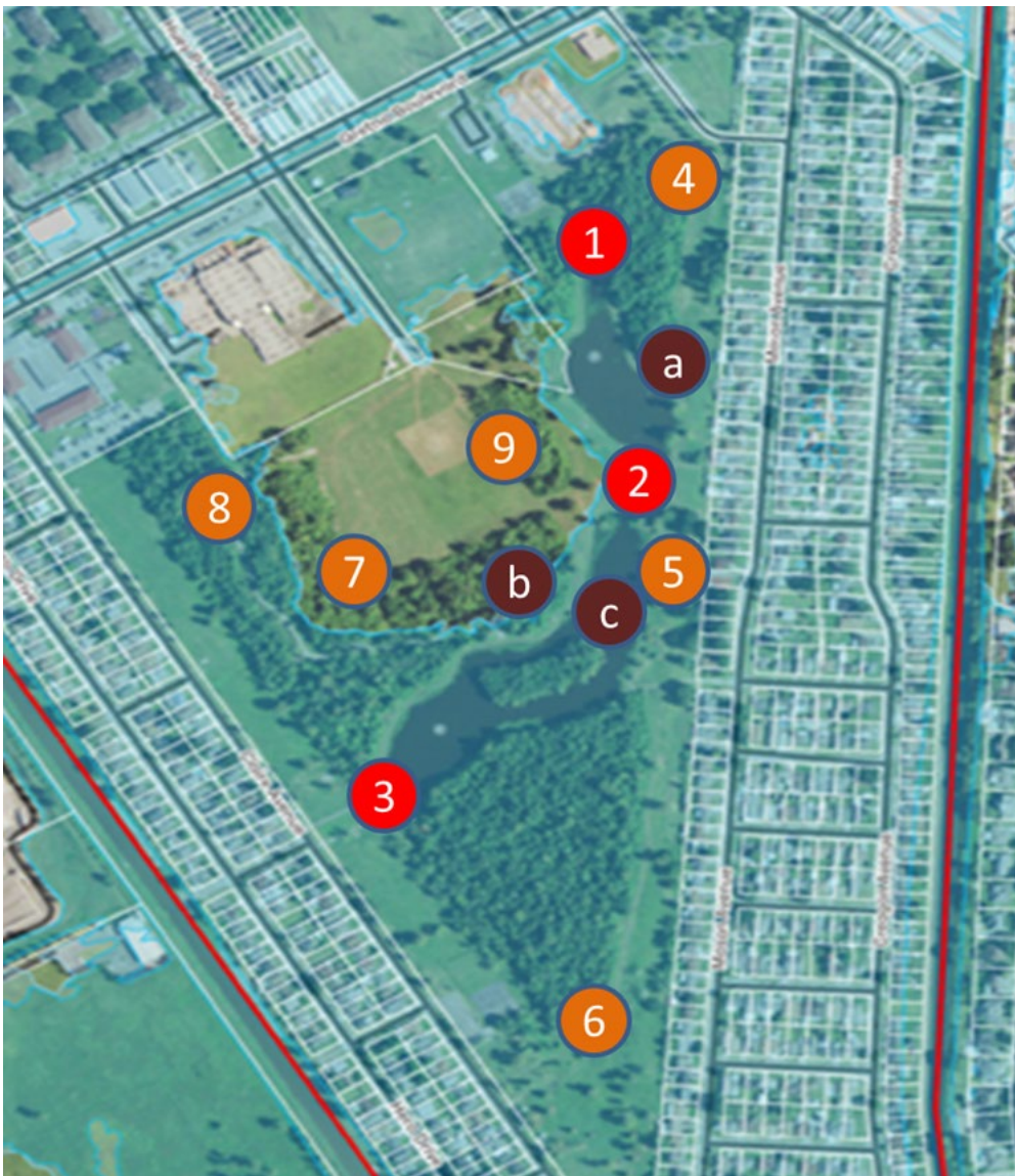
Figure 1: Proposed monitoring locations. Red: surface water level and quality monitoring locations; Brown: groundwater surface water interaction monitoring locations, Orange: groundwater observation well.
